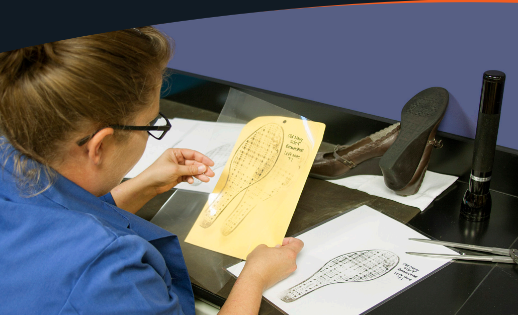
Darian Stinson, with the Missouri State Highway Patrol Crime Laboratory, using a transparency overlay technique for direct comparison of footwear impressions
